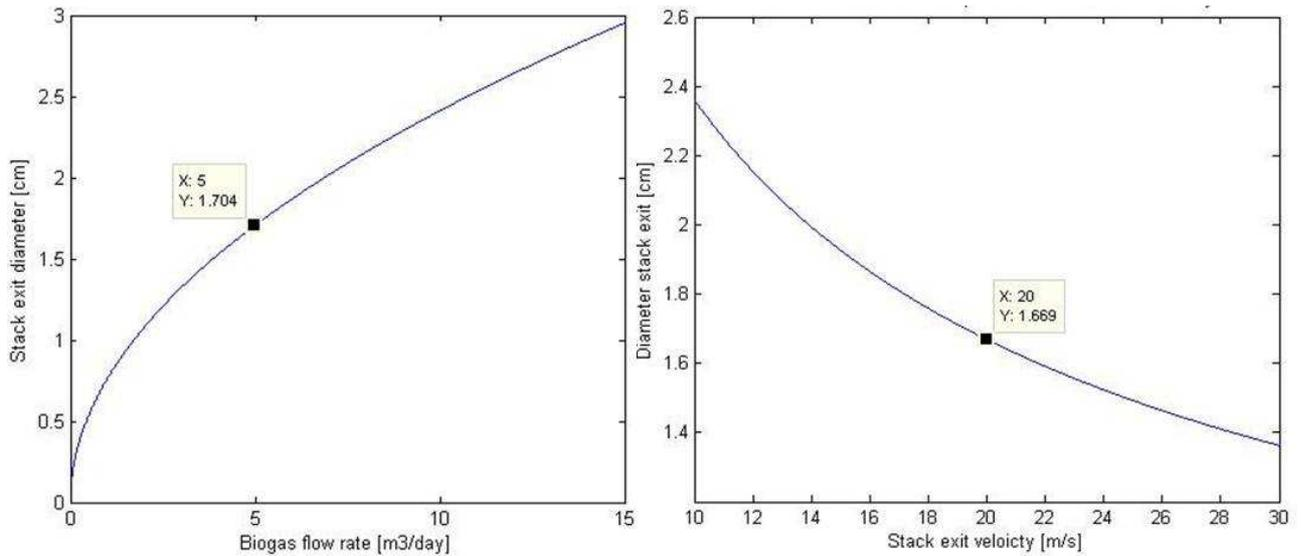
**Figure 10: The stack exit diameter as influenced by the biogas flow rate (left) and the stack exit velocity (right)**
