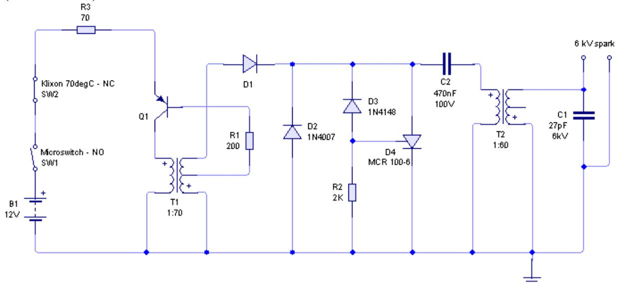
**Figure 20: Scheme of the electronic setup for the combination of microswitch, klixon and spark ignition**
