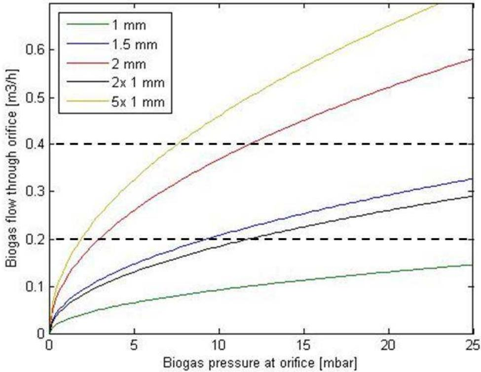
**Figure 8: Theoretical biogas flow rate through orifices with  $C_d$  is 0.75 and lines indicating biogas production of 5 and 10  $m^3/day$**
