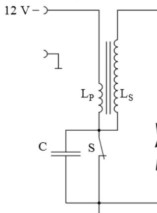
**Figure 17: Scheme of the electronic principle of a car bobbin (Wikipedia 2012b)**
