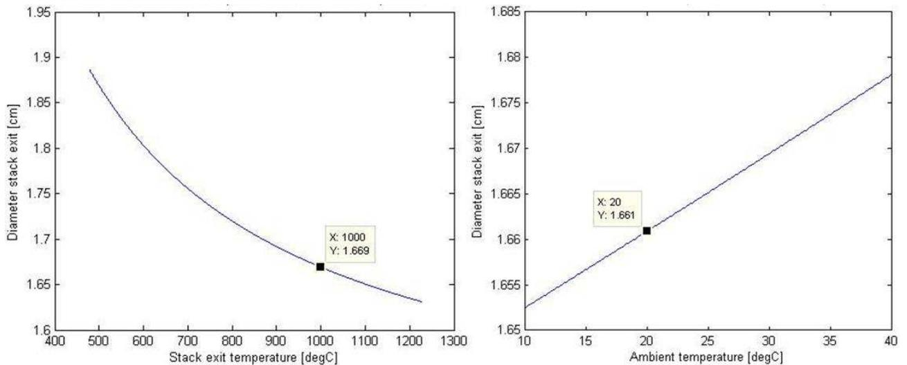
**Figure 11: The stack exit diameter as influenced by the gas temperature (left) and the ambient temperature (right)**
