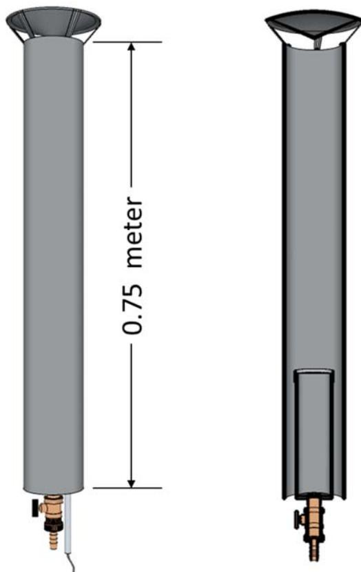
**Figure 28: Side view and cross section of the flare enclosure and hood**
