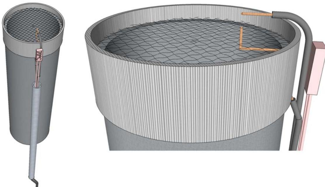
**Figure 27: Fixation of ignition system, temperature switch and cables to mixing tube and burner head**
