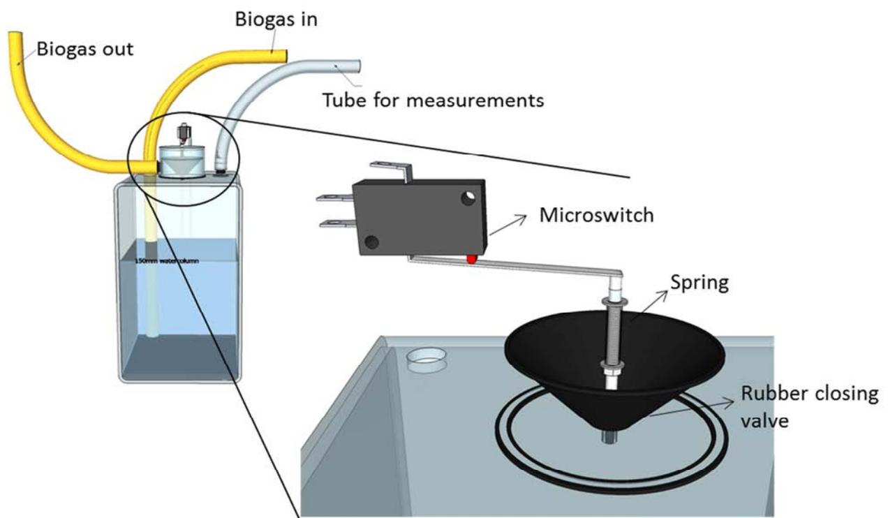
**Figure 15: Drawing of the pressure monitor and gas valve with details of valve and microswitch**
