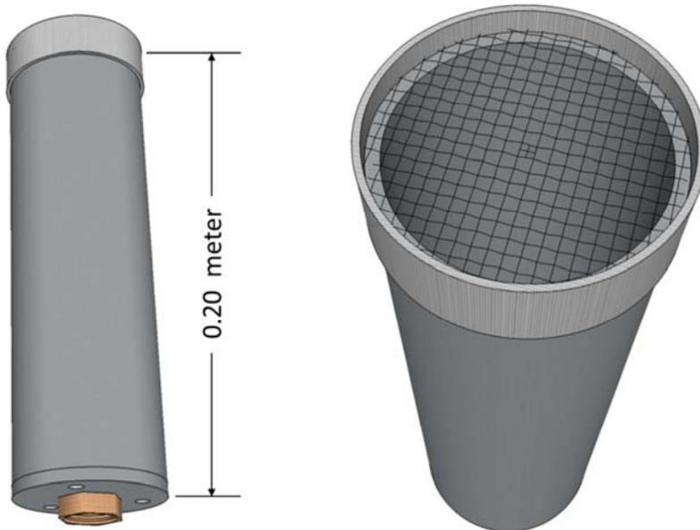
**Figure 26: Side and top view of the mixing tube and burner head**
