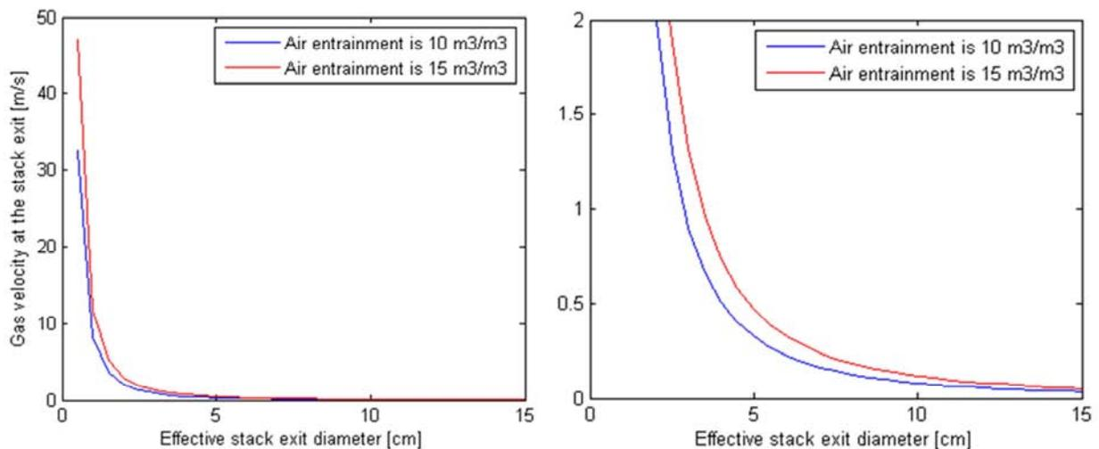
**Figure 13: The influence of the diameter of the stack exit and the air entrainment rate on the gas velocity**
