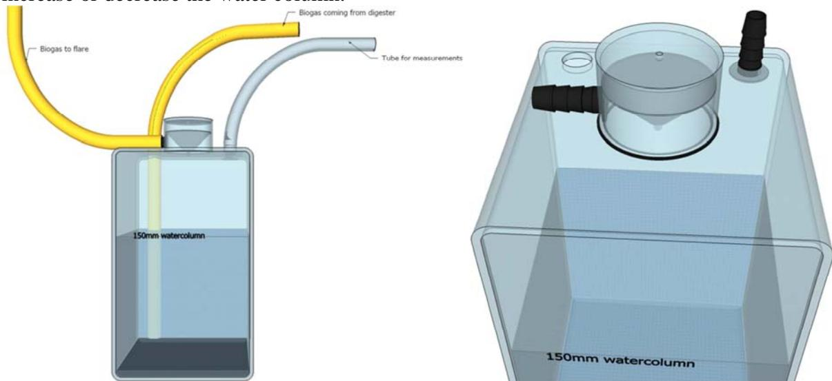
**Figure 23: Drawing of pressure monitoring, gas valve and tubing**
