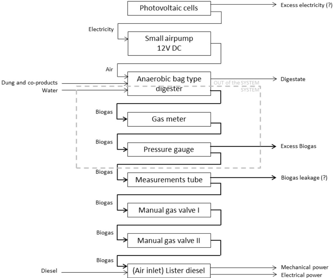
**Figure 3: Process chart of the biogas production system in Koulikoro, Mali (determined from video produced by FACT)**
