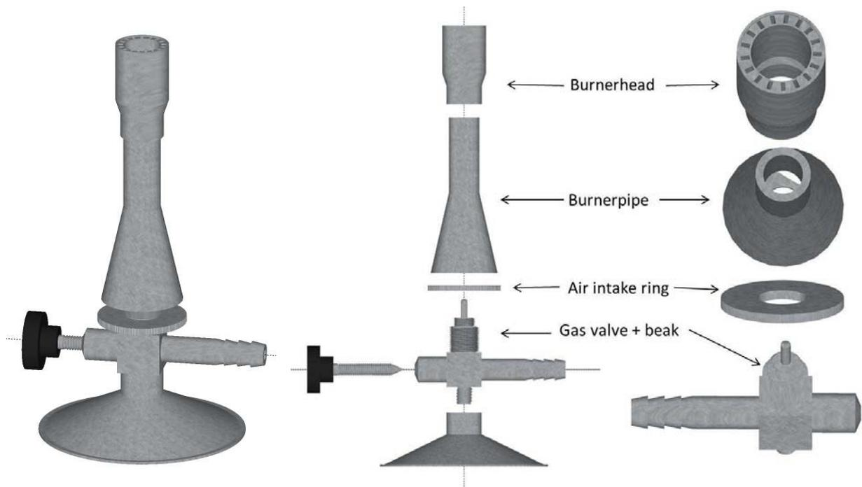
**Figure 4: Bunsenburner (complete at left, disassembled at right) as used for preliminary testing**
