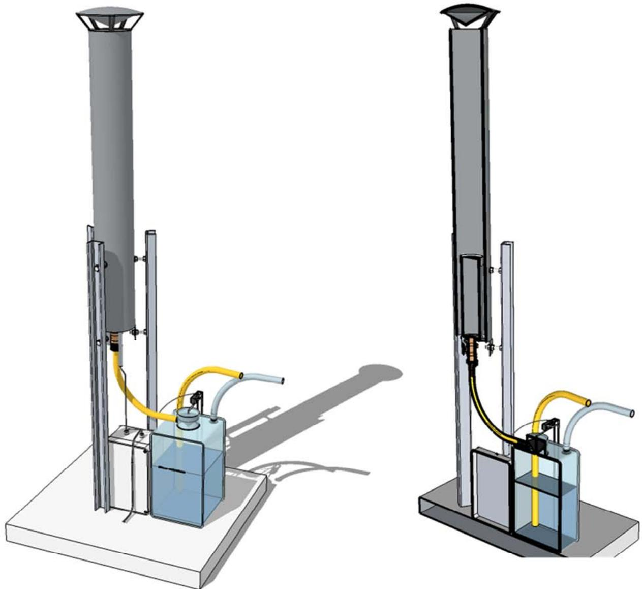
**Figure 30: Overview and cross section of the complete flaring system**
