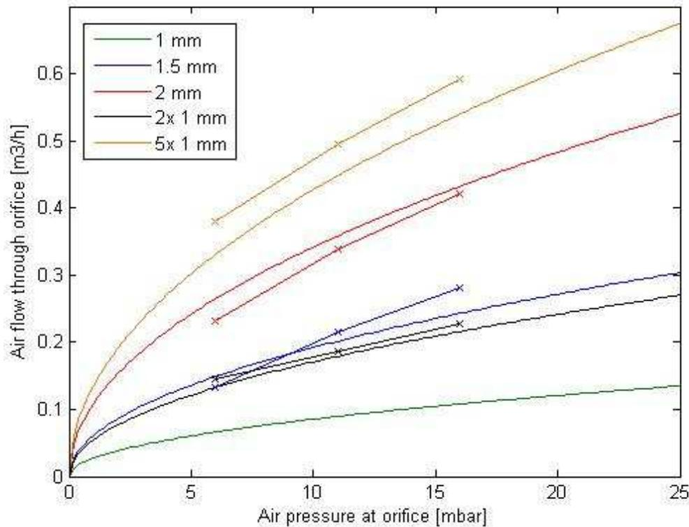
**Figure 7: Theoretical and measured (+) flow rates through orifices for air with  $C_d$  set to 0.75**
