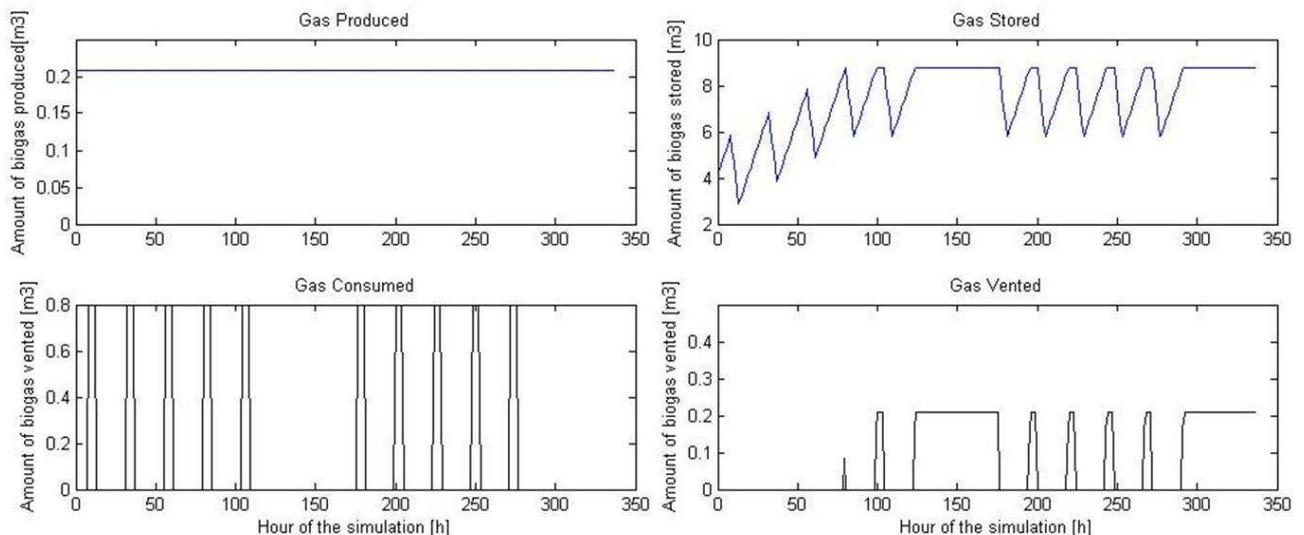
**Figure 21: Hourly biogas production, consumption, amount of biogas in storage and vented for scenario 1**
