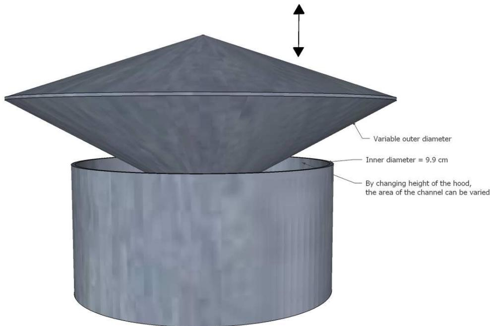
**Figure 14: The surface area of the enclosure can be chosen by varying the distance between hood and enclosure**
