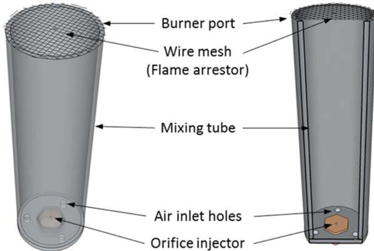
**Figure 9: Drawing of the setup used for testing of the port dimensioning**
