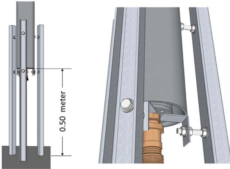
**Figure 29: Flare support construction**
