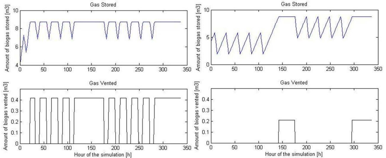
**Figure 22: Hourly prediction of the amount of biogas stored and vented for scenario 2 (left) and scenario 3 (right)**
