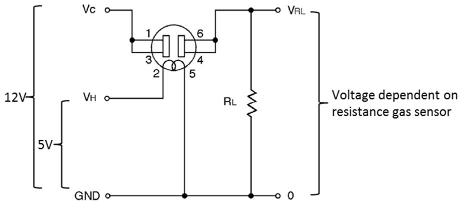
**Figure 16: Basic scheme of the Figaro TGS-813 gas sensor (Figaro 2012)**
