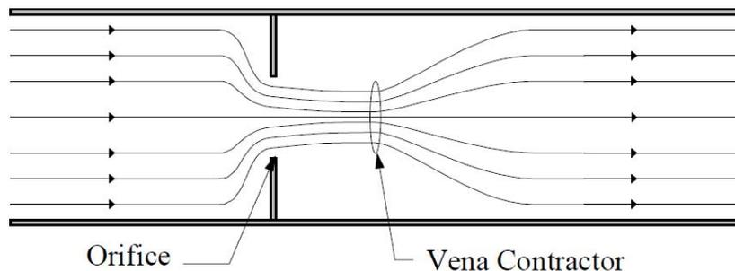
Figure 6: Schematic image of an orifice in a tube (Fulford 1996)
