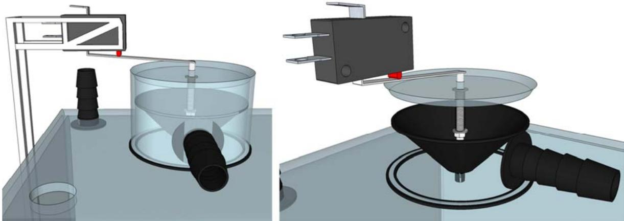
**Figure 24: Spring loaded gas valve with microswitch and details of the spring loaded valve**
