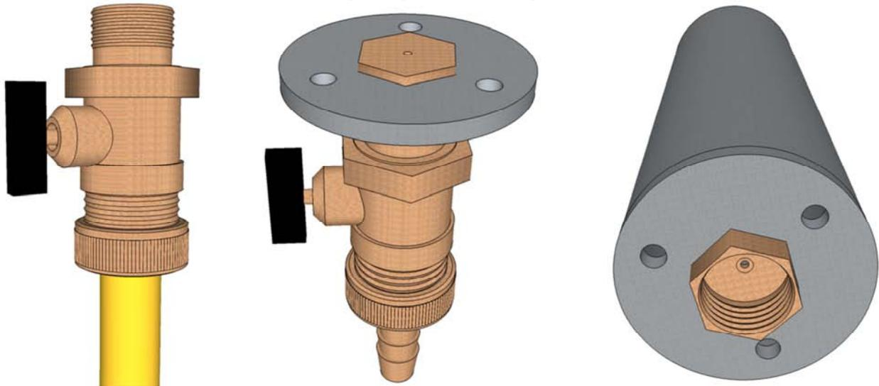
**Figure 25: Manual gas valve, orifice and primary air holes (left) and cap with injector orifice, air holes and mixing tube (right)**
