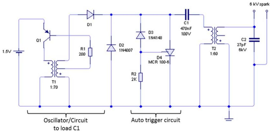
Figure 18: Scheme of the 1.5 Volt spark generating circuit (Ridders 2012)
