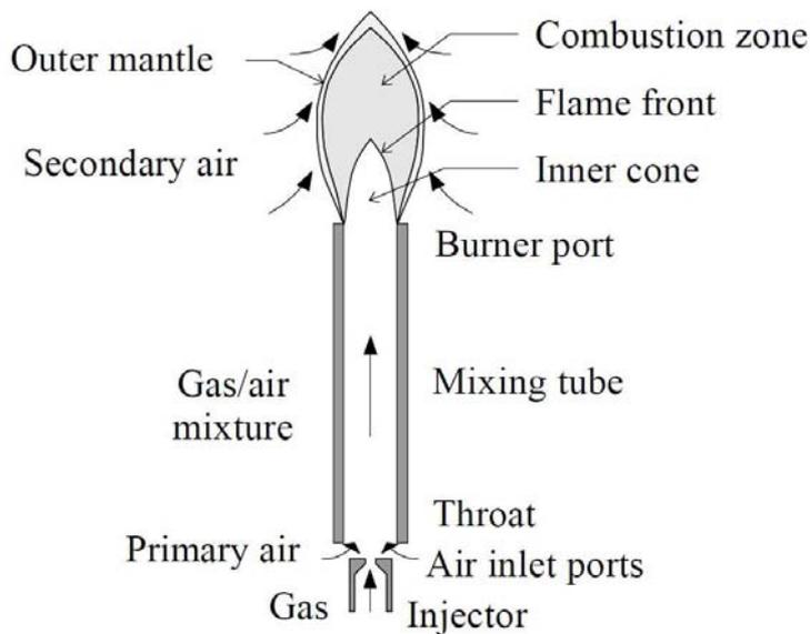
Figure 5: Schematic drawing of the elements of burner and flame (Fulford 1996)
