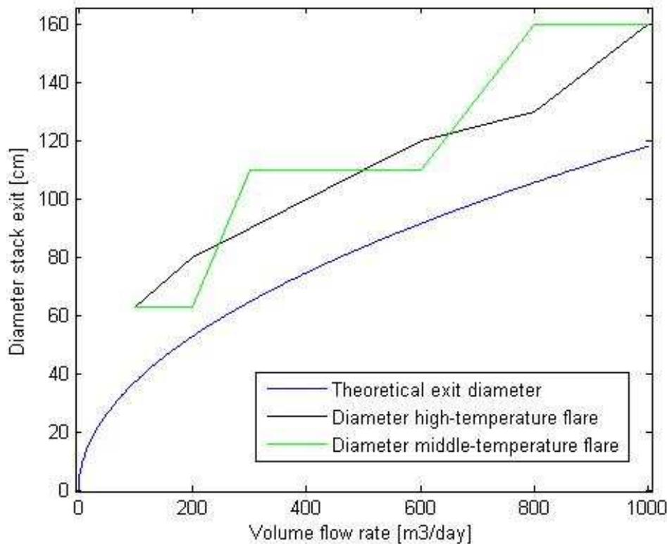
**Figure 12: Comparison of theoretical values for the stack exit diameter and dimensions of flare stacks of Himmel Gastechnik**
