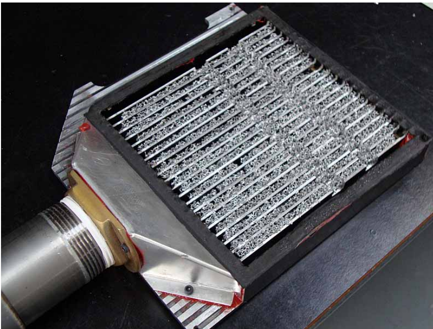
Figure 11 Aluminium foam pressed between the hex fins
